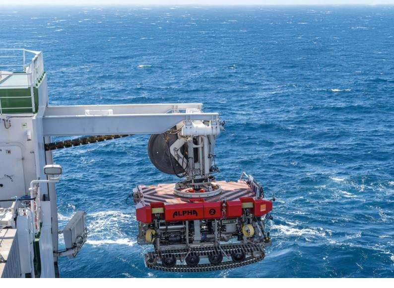
Alpha is a powerful and full customized work class ROV dedicated for cable (energy and telecom) and pipes works (burial, survey, inspection).
