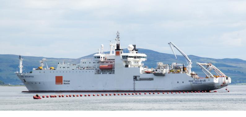
Tailored-built for Orange Marine in 2002, cable ship Descartes is a versatile, high technology vessel, designed to lay and repair submarine fibre optic systems.
