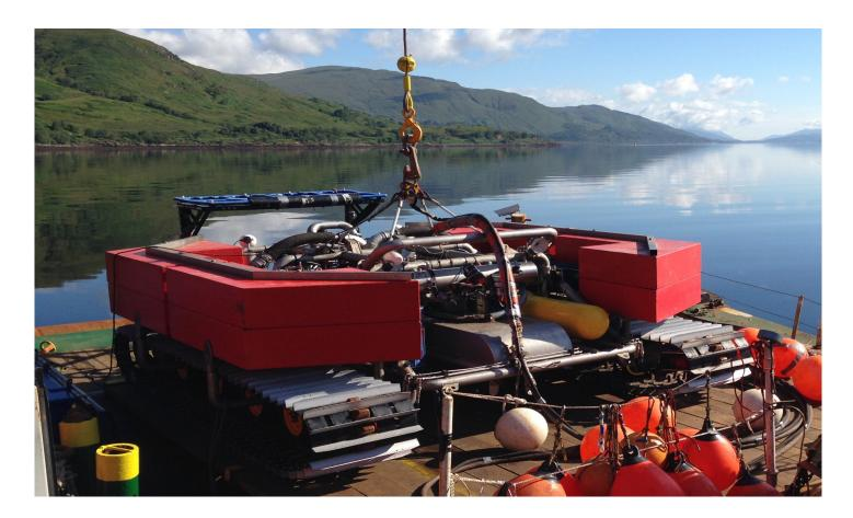
J-Swoc is a powerful Jetting Crawler dedicated for shallow water cable works. This product is design to bury all kind cable or pipes up to 200mm diameters from the shore up to 100m. The J-Swoc is fully instrumented and avoids a burial by divers or jetting sledge with a high level of quality and efficiency.
