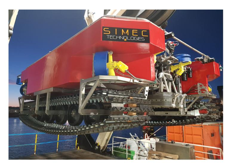
SEAGMA is a light and powerfull trenching ROV able to bury cables (power and telecom), O&G umbilicals and pipes. Its full instrumentation package allows also inspection and survey operations with a high level of performance. This trencher is customizable to meet the customer requirements and project specificities.
