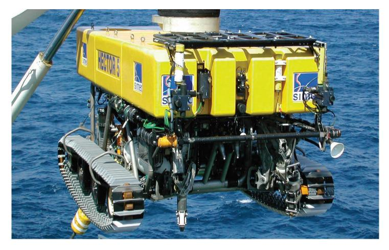
Hector is a powerful and full customized work class ROV dedicated for cable works and designed to fullfil customers specifications for quality protection of submarine cables, umbilicals or flexible pipes. Those products have demonstrated theirs qualities during 12 years of experience all around the world. During this period SIMEC built 7 units of Hector upgrading each time the efficiency and the maintainability of these ROVs.
