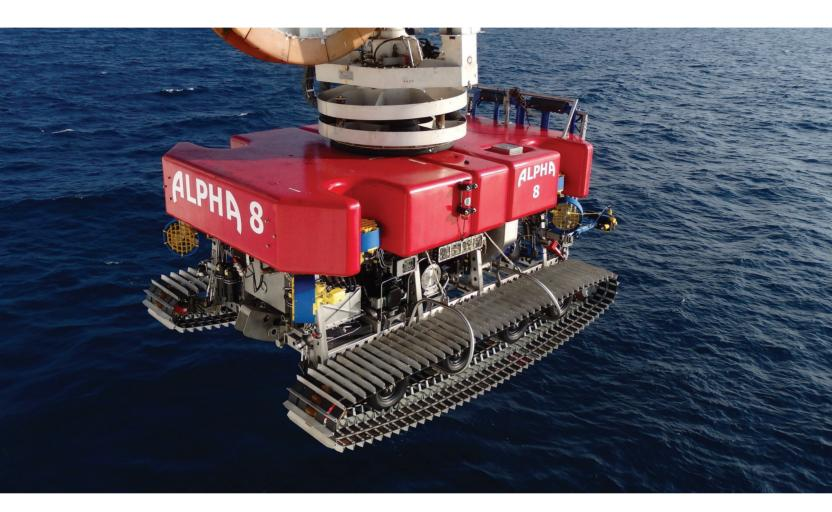
Alpha 8 is a powerful and full customized work class ROV dedicated for cable (energy and telecom) and pipes works (burial, survey, inspection).
