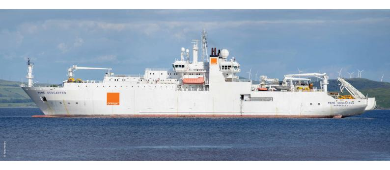
Tailored-built for Orange Marine in 2002, cable ship Descartes is a versatile, high technology vessel, designed to lay and repair submarine fibre optic systems.
