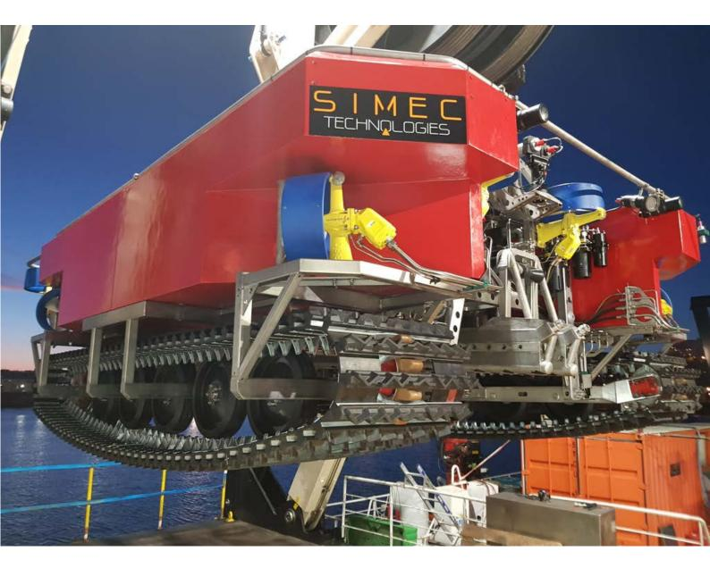
SEAGMA is a light and powerfull trenching ROV able to bury cables (power and telecom), O&G umbilicals and pipes. Its full instrumentation package allows also inspection and survey operations with a high level of performance. This trencher is customizable to meet the customer requirements and project specificities.
