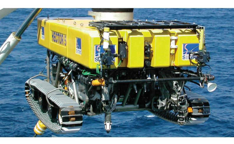
Hector is a powerful and full customized work class ROV dedicated for cable works and designed to fullfil customers specifications for quality protection of submarine cables, umbilicals or flexible pipes. Those products have demonstrated theirs qualities during 12 years of experience all around the world. During this period SIMEC built 7 units of Hector upgrading each time the efficiency and the maintainability of these ROVs.
